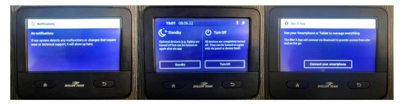
The notification sceen will show any notifications and error messages The turn off button gives you the option of switching to standby, or turning the panel completely off. The iNet-X App button starts the process of connecting your smart phone using the iNet-X ap.
