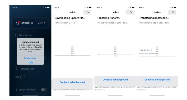
If you get a notification to update your firmware, follow the process through downloading, preparing and transferring the file using the iNet-X app on your smartphone, then installing the firmware update using your panel.
