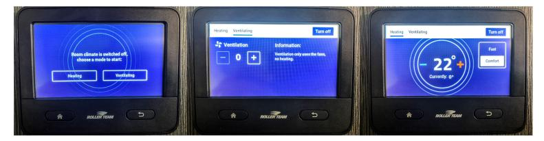
Room climate gives you the option of choosing between fresh air ventilation by adjusting the fan speed, or adding heat by adjusting the desired temperature.
